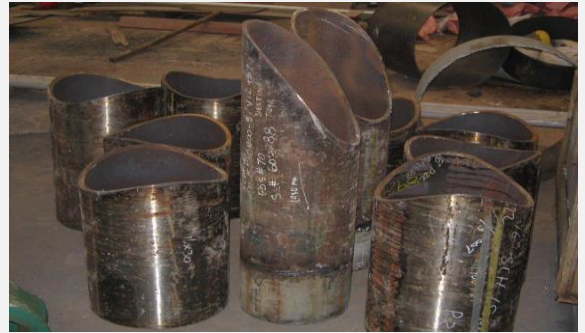
Fabrication Pipe Nozzles
