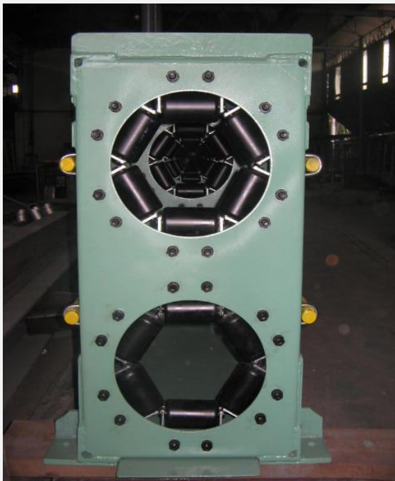
Shop Fabrication Pipebelt Conveyor Coal Boiler Project
