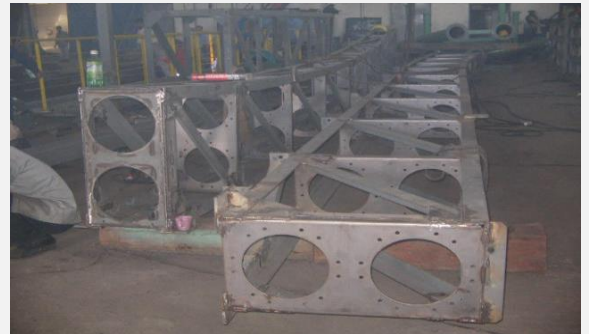
Shop Fabrication Pipebelt Conveyor Coal Boiler Project
