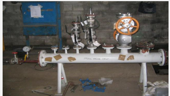
Pressure Test for Valves
