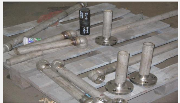
Fabrication Spool Pipe for Sealing PU-5207-AB at PT.
